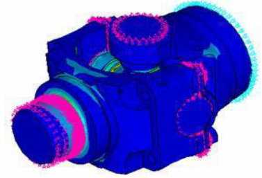
Example of MPC Bonded Contact to Connect Different Regions in an Assembly.
